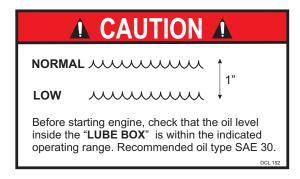
Figure 17. Lubrication Box Oil Caution Decal
